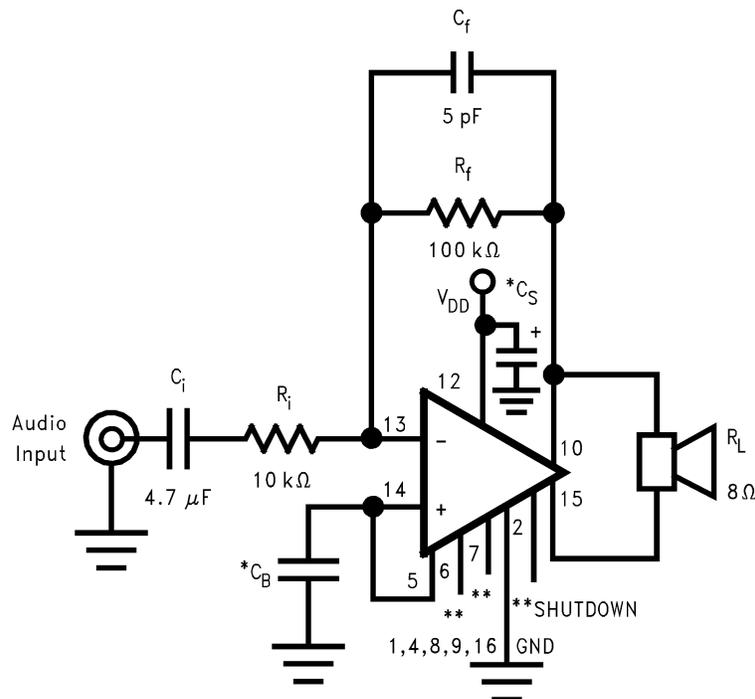
Figure 3. Stereo Amplifier with  $A_{VD} = 20$
