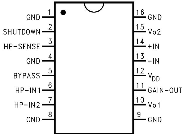
Figure 2. SOIC Package- Top View
