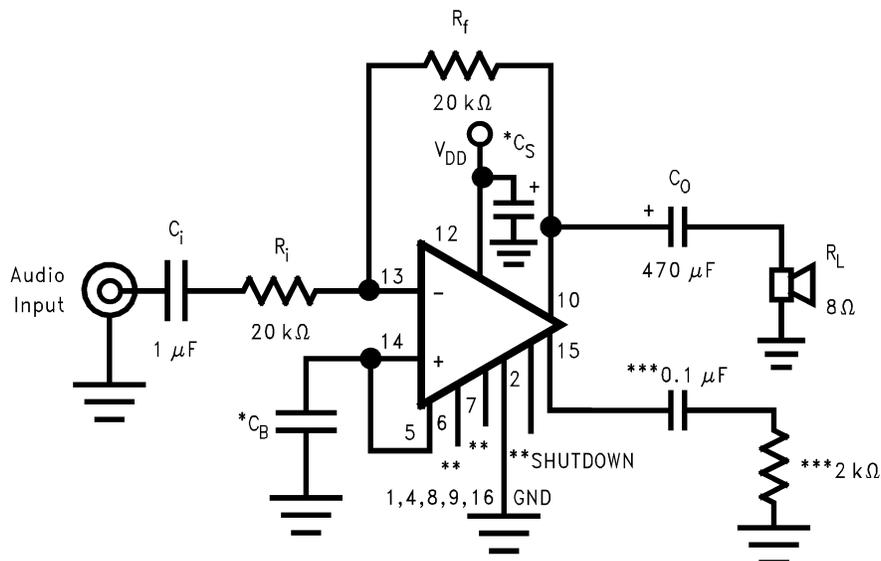
\* $C_S$  and  $C_B$  size depend on specific application requirements and constraints. Typical values of  $C_S$  and  $C_B$  are  $0.1 \mu\text{F}$ .
