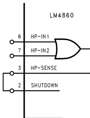
Figure 21. HP-SENSE Pin to SHUTDOWN Pin Connection
